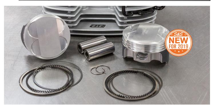
These high compression pistons feature a 7cc raised dome to achieve a compression ratio of 11:1 (from 9.5:1). Higher compression is a key factor in increasing performance.
