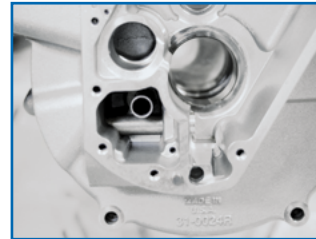
Relocated oil scavenger pick-up reduces oil carry-over by increasing oil scavenger efficiency.
