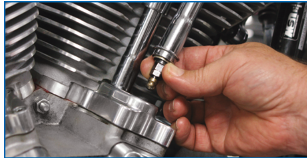
When a Quickee adjustable pushrod is collapsed, it can easily be installed or removed from an assembled engine.
