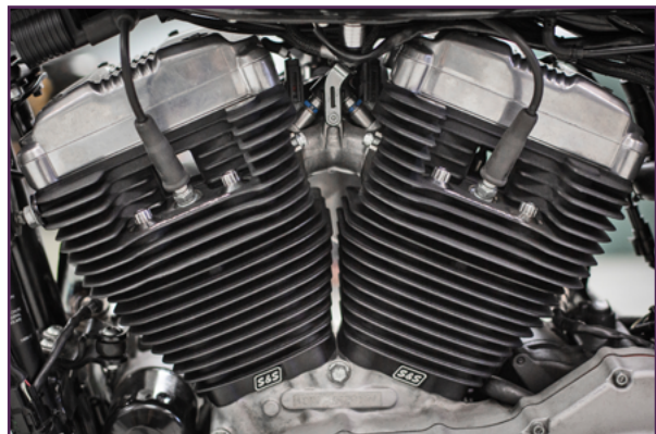
S&S cylinders match the fin profile on 1986–'03 cylinder heads. Although there is a slight difference in the fin profiles of S&S cylinders and stock 2004–'20 cylinder heads (shown above), the look is generally not considered to be objectionable. You decide!
