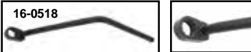
Left Rear Engine Mount Bolt Wrench allows removal and installation of left rear motor mount bolt on Big Twins without removing the inner primary cover. VT No. 16-0518
