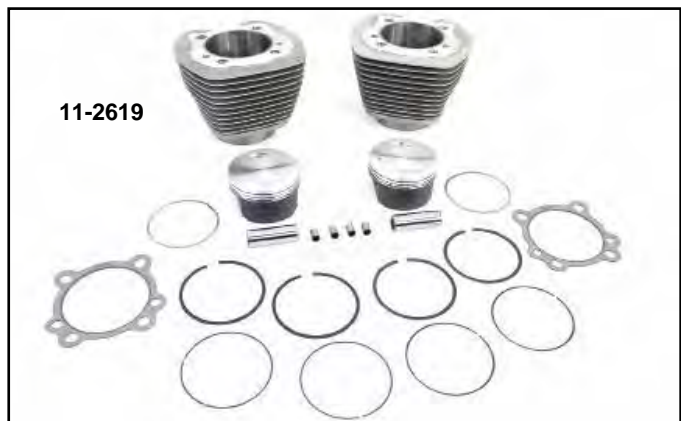
Twin Cam 3 \frac{7}{8} " Big Bore Cylinder Kit increases displacement of Twin Cam 88 (1450) to 95 cubic inches (1550). These cylinders require no crankcase machining and are finished honed.
