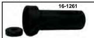
Transmission Main Drive Gear Nut Wrench Tool. Use to remove the 2 1/4" hex nut from main drive gear which secures the rear drive trans pulley. Use with 1/2" drive ratchet. Use on all 2006-up Dynaglide and 2007-up FXST-FLT models. VT No. 16-1261 Brand Sifton
