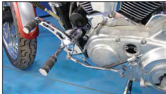
1986-03 Billet Forward Control Kit features Big Twin style controls. Order related brake parts separately. Kit will not work with stock exhaust. VT No. 22-0790
