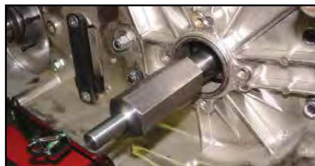
4-Speed Transmission Arbor replaces clutch hub nut to allow test rotation with 1/2" drill. VT No. 16-1274
