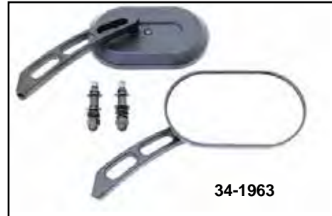
Billet Mirror Set feature oblong shape and slotted stem to fit 1982-up control handles, sold in pairs.
