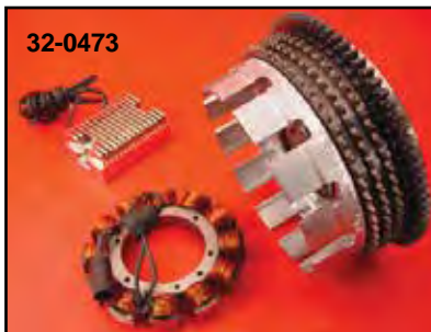
Charging System Kit for XL's developed by V-Twin in 1995
