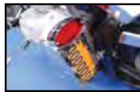
31-0891 bracket use to mount 33-0588 Lamp assembly on 2007 Softail or 2006-up FXD
