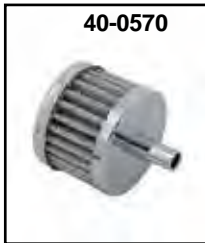
Chrome Crankcase Vent clamps direct to 3/8" breather hose. Unit comes with a 5/16" stud and nut or 1/4" x 20 threaded insert to mount from bracket. Measures 2" diameter x 1 1/2" high.
