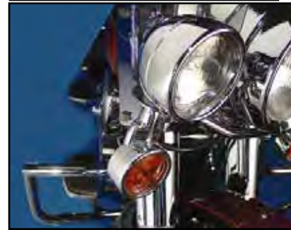
VT No. 33-0578 Frenched Turn Signal Trim Ring Kit includes chrome plated rings fit front or rear on 1988- up FLT and FLST models. VT No. 33-0578
