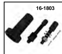
Big Twin Mainshaft Seal Remover and Installer replaces 95660-42. Use to install and remove main seal. This tool will push seal in as flat and straight as possible to .050 below housing for a no leak fit. VT No. Years Speed 16-1803 1936-76 4 16-0700 1985-up 5
