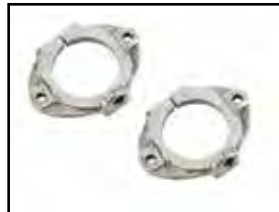
Wide Glide Fork Cover Tab Set constructed of raw cast steel. Set is for both sides of Wide Glide FLH triple trees. Tabs accept stock fork covers or cowl set on 1949-1984 FL models. VT No. 24-1431
