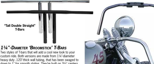
custom ride. Both versions are made from 11/4"-diameter heavy duty .120"-thick wall tubing, that has been swaged to down to 1" for smooth styling. They're built on 3½" centers and come pre-drilled for easy internal wiring of all OEM type controls from 1982 to present (except electronic throttleby-wire models).
