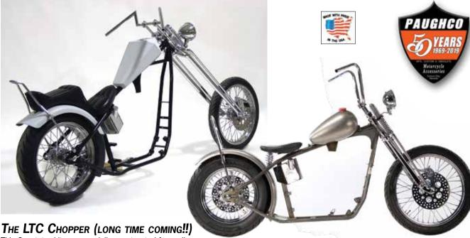
This Sportster kit was specially-constructed from all of our best selling parts to create this iaw dropping custom Chopper. An industry first, this rolling chassis kit features a wide tire frame with 3" out and 6" up, and a 40° neck rake. A beautiful 18" over tapered leg Springer with shock and brake mounts is included, as well as the wheels, tires, front brake and rotor, headlight, handlebars, risers, oil tank, rear fender,
